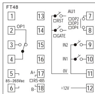
OP1 relay 5A/250Vac(resistive load)
